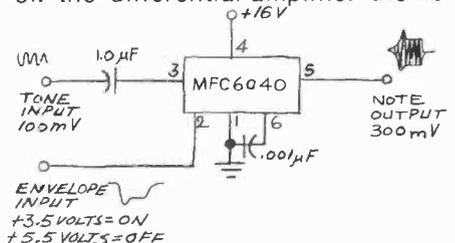
Fig. 5. Gain block envelope shaper.
