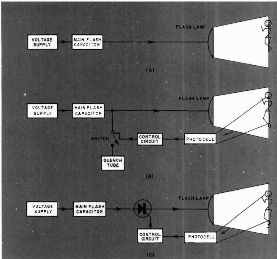
Three greatly simplified block diagrams show the major components of the various types of electronic flashers. At (A), a manual unit is the least complex. Diagram (B) shows how a photocell is added with control circuit and quench tube to dump surplus energy. At (C), a thyristor unit adds an SCR to trap voltage from the main flash capacitor.
