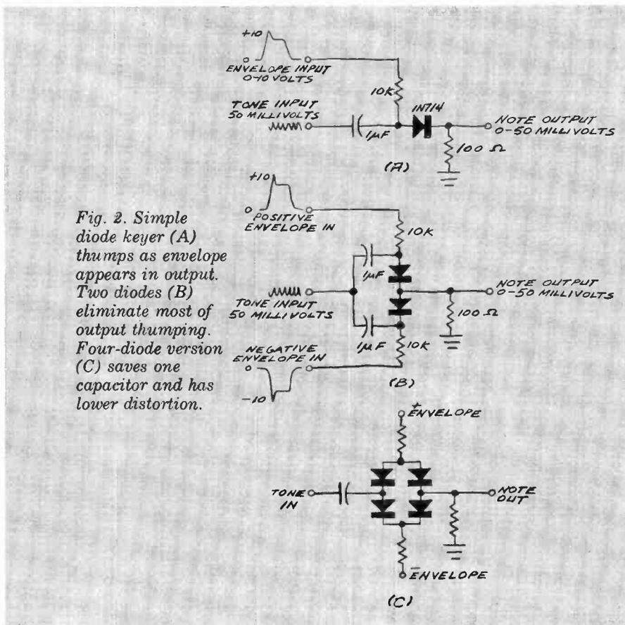
Fig. 2. Simple diode keyer (A) thumps as envelope appears in output. Two diodes (B) eliminate most of output thumping. Four-diode version (C) saves one capacitor and has lower distortion.
