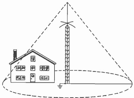
Fig. 3. A metal antenna tower, properly grounded, provides a cone of protection for the house.
