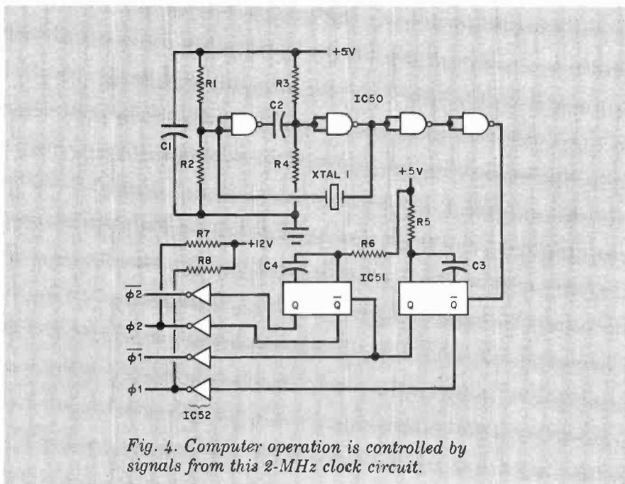
Fig. 4. Computer operation is controlled by signals from this 2-MHz clock circuit.
