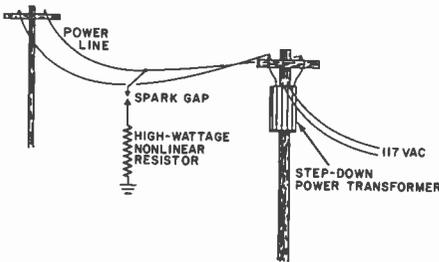
Fig. 2. In power-line arrester, current is reduced by resistor.
