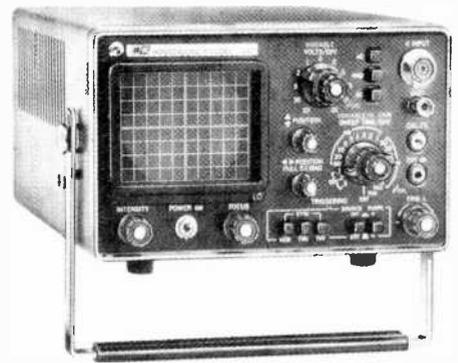
available. Rise time of the vertical amplifier is 35 nanoseconds, overshoot is 3% or less, and the input impedance is 1 megohm shunted by 35 pF. The 1431 is supplied with a handle/tilt stand, Mylar vector overlay (so the unit can be used as a vectorscope), but less probe. It is \$399.00.
