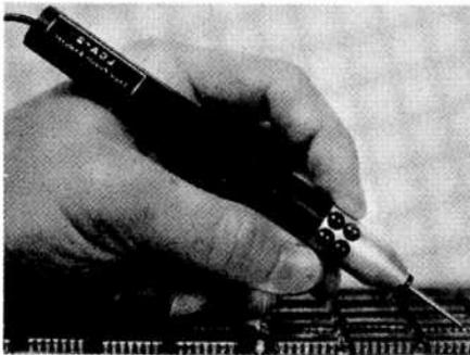
input. The LCA-2 is supplied with a 4-foot coaxial cable, BNC connector, and three input adapters. It can indicate polarity/duty cycle of pulse trains as high as 25 MHz. The probe measures 5½-in. long and ⅝-in. in diameter. \$69.50.
