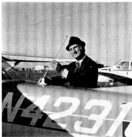
Antenna, on plane's fuselage, is cut for channel 13.
