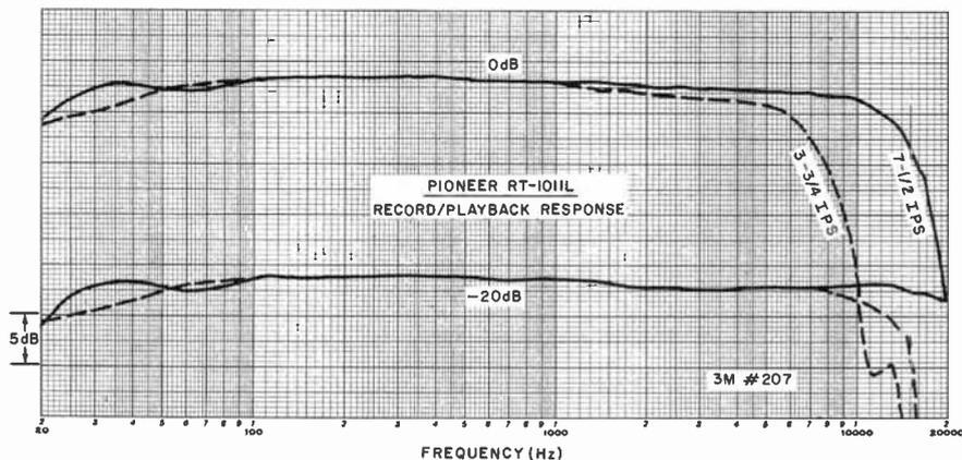
order to be very accurate at both speeds. It was within  $\pm 0.5$  dB from 50 Hz to 15,000 Hz at  $7\frac{1}{2}$  ips and within  $\pm 0.8$  dB from 50 Hz to 7500 Hz at  $3\frac{3}{4}$  ips. (These are the frequency limits of the test tapes.)
