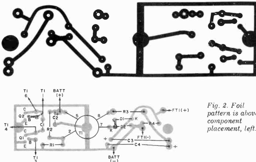
Fig. 2. Foil pattern is above, component placement, left.
