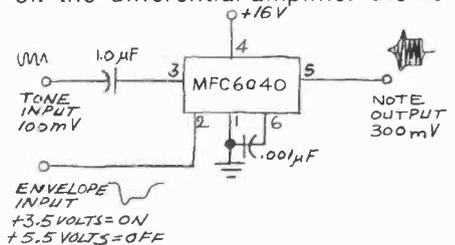
Fig. 5. Gain block envelope shaper.
