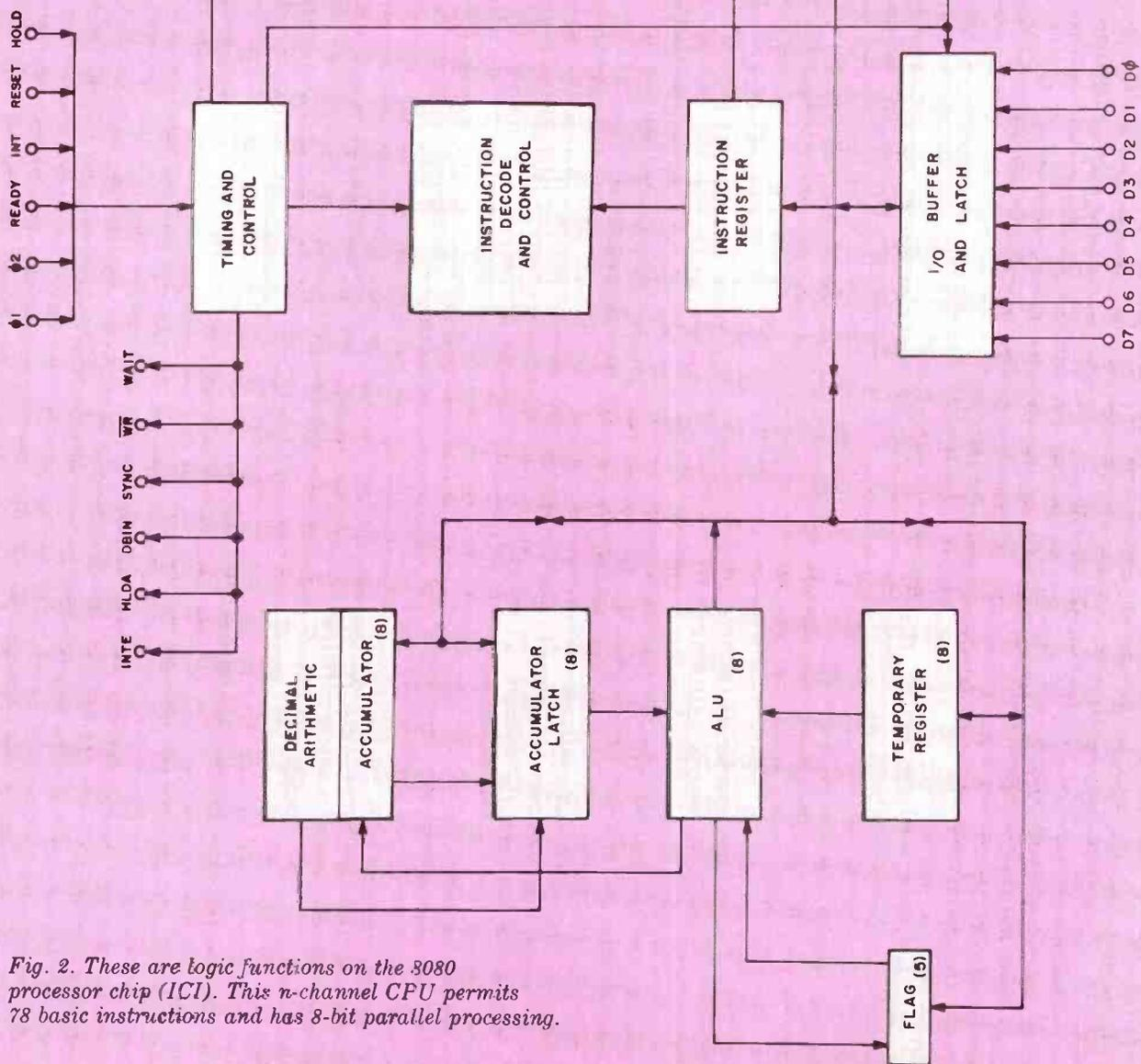
Fig. 2. These are logic functions on the 8080 processor chip (IC1). This n-channel CPU permits 78 basic instructions and has 8-bit parallel processing.
